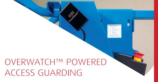
An Anti-Entrapment Secondary Guarding Device For Scissor Lifts, Ensuring Users Are Safe From Obstructional Hazards...
