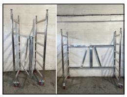
**1.** Ensure all castors are firmly fitted to the folding frame. Then open folding frame and engage toggle clamps. When fitted with adjustable legs, level your tower using a spirit level as a guide.
