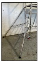
**4.** Fit your 4 stabilisers as early as possible. Use the diagram on page 5 for the best stabiliser positioning.
