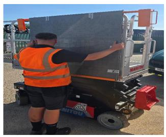
• Slide both side extenders inward until the materials are within the cup bracket of the extender arm and positioned so that materials cannot slip out.
