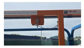
• Line up the lower rail brackets and slide the extender down until contact is achieved.
