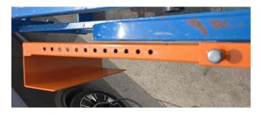
The plunger type pins are pictured below and when the sliders are correctly latched will sit fully down. Images below show unsecured (I) and secured (r)
