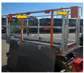
• Standing outside of the platform, carefully lift materials onto the trough. Ensure that all materials are within the trough tray.
