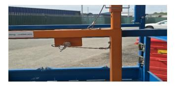
• Ensure that the upright rail holes are visible on both sides of the attachment and insert locking pins.
